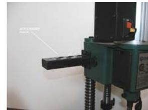
Install the fence through the round opening above the wood base, slide the large spring on the fence shaft between the back of the fence and the lock-down lever.
