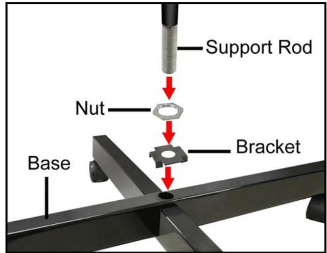
Figure-3 Attaching the bracket, nut and support rod
