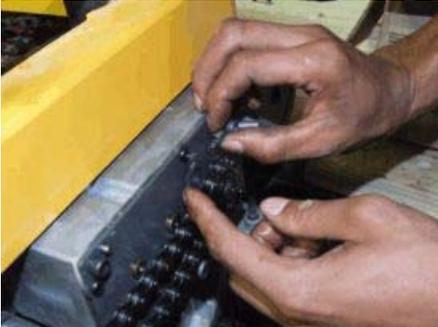
**17. Remove the chain and sprockets together.**
