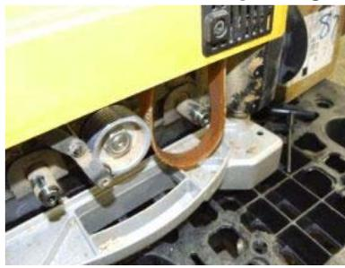
**11. Remove the nut and washer from the end of the head.**
