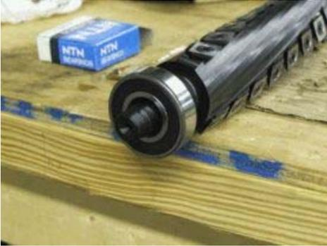
**24. Carefully slide the new head through the bearing housing. Be careful of alignment so as not to bind the carbide knives and chip or break them.**
