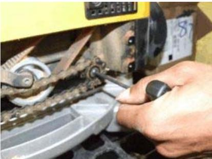
**9. Remove the chain and sprockets together.**
