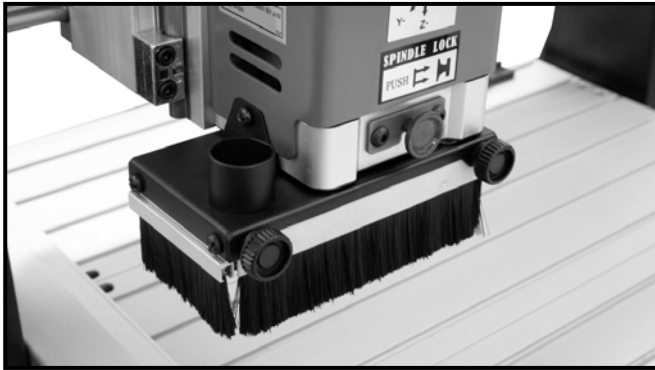
Figure-1 Installing the collection skirt
