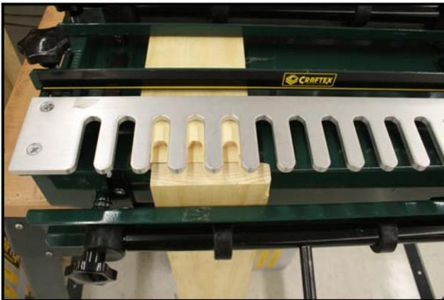
*Figure 11 shows dovetails after cutting*
