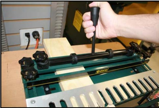
*Figure 5 shows clamping down the work-piece*
