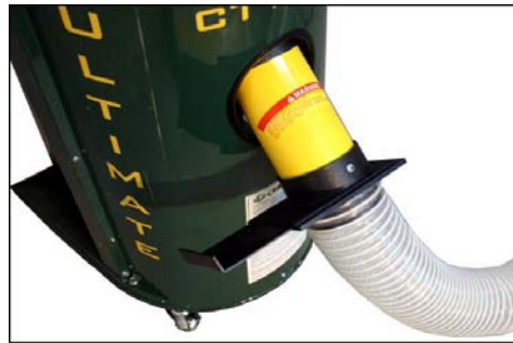
Open the top blast gate to allow air flow from desired tool.
