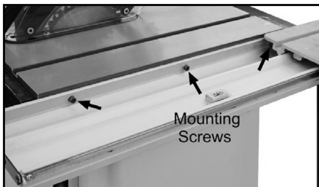
Figure-5 Installing the sliding table
