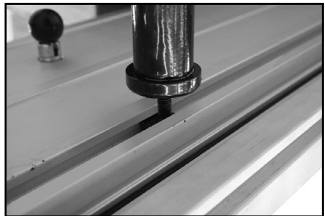
Figure-3 Attaching the support leg to the sliding table
