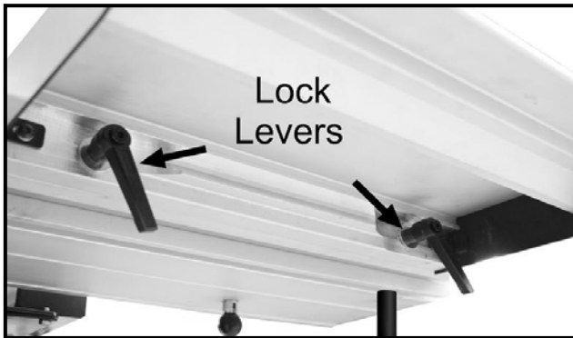
Figure-7 Installing the extension table
