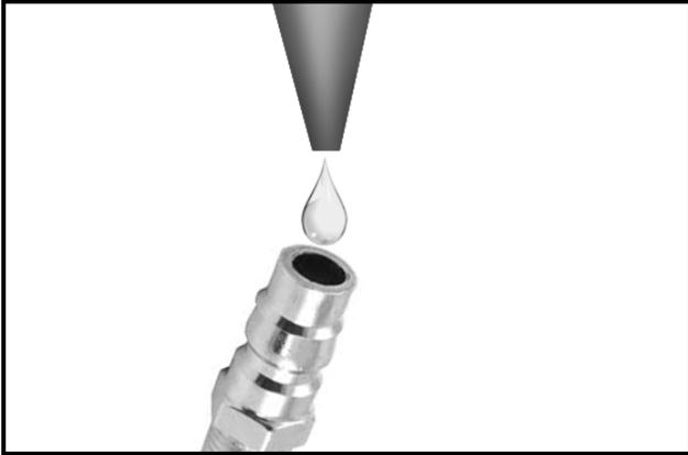
Figure-2 Lubricating the stapler
