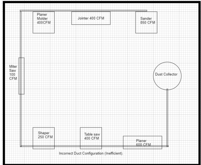
Figure 5: Incorrect system configuration.
