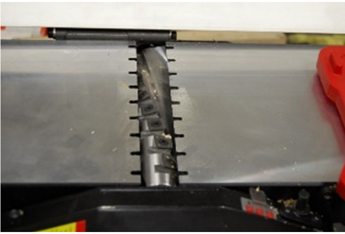
Figure 30b: The cutterhead exposed ready for insert replacement
