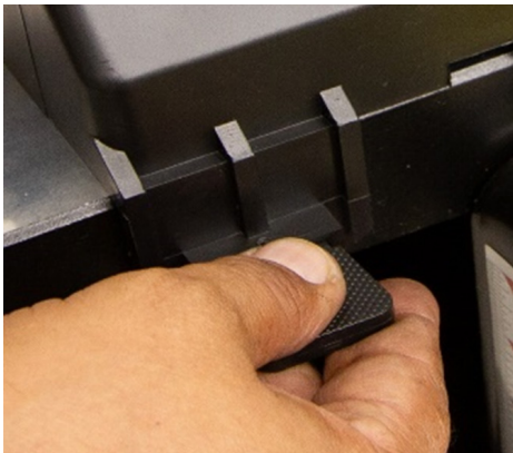
Figure 7: Dust Port and interlock Keys installed.
