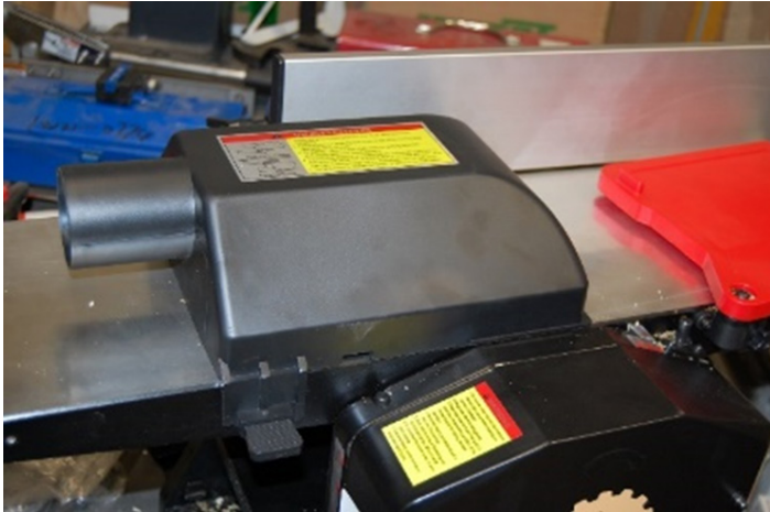
Figure 25: the dust hood is secured for planing operation.
