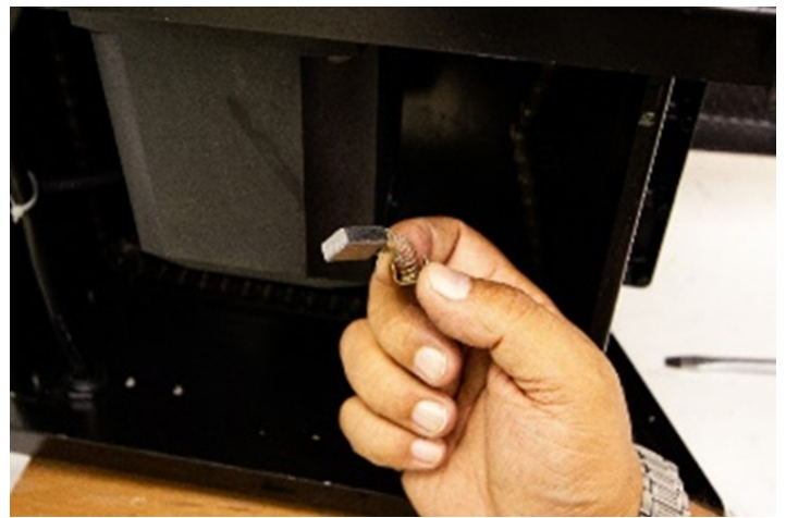
Figure 45: Motor Brush replacement.
