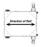
A short narrow base, such as found on a drill press or bandsaw, may benefit from this arrangement. Due to swivel rotation base may sit out of level. Rotate swivel wheel away from base to correct.
