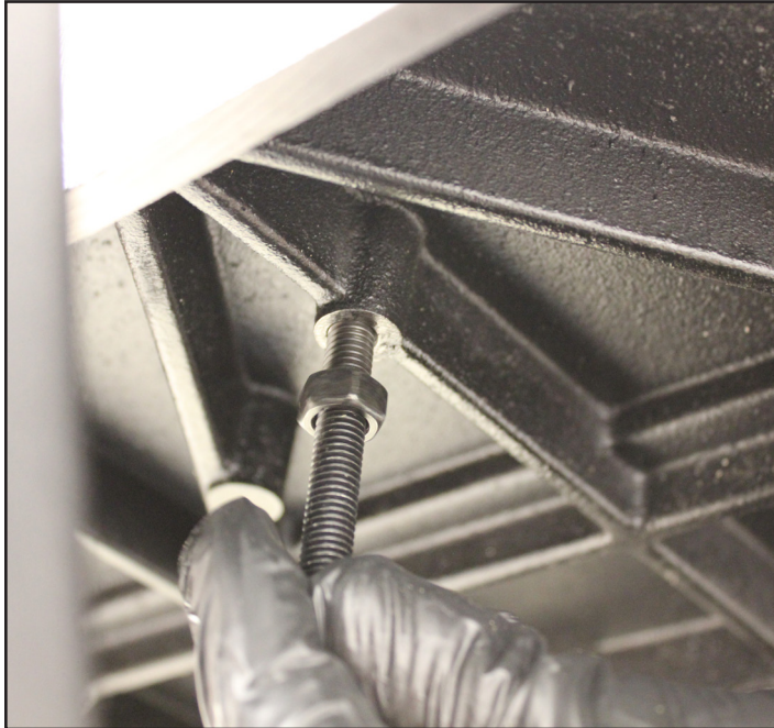
Figure 9: Installing the 90-degree table stop.
