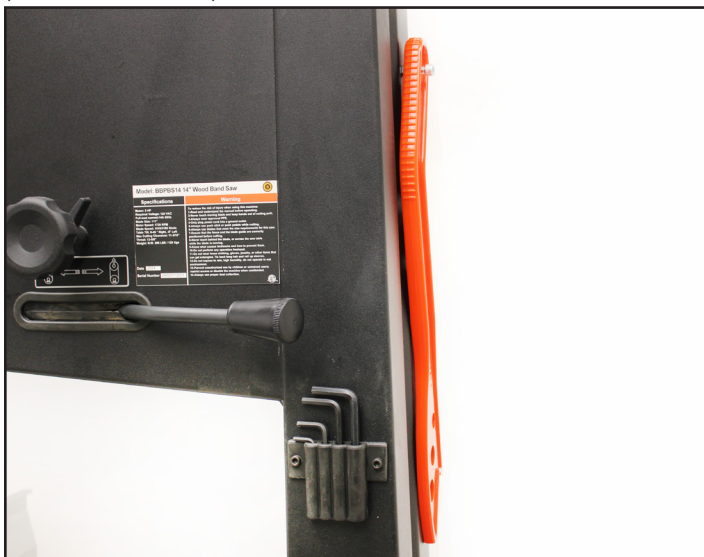
Figure 13: Installing the tool and Push Stick Holders.
