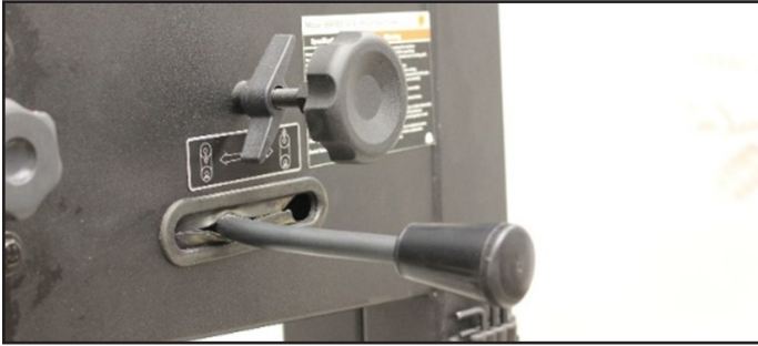
Figure 19: Blade Tracking mechanism.
