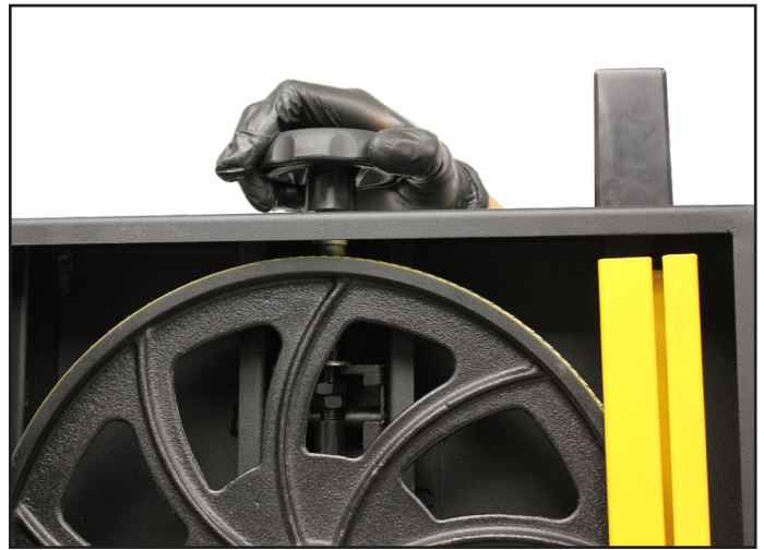
Figure 20: The Blade Tensioning Handwheel.
