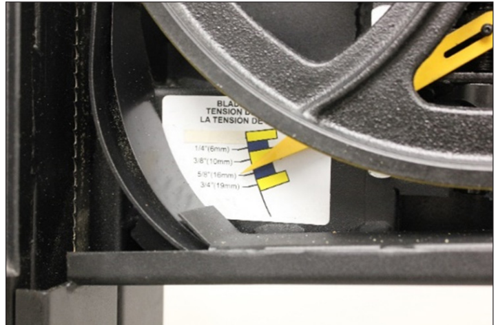
Figure 21: The Blade Tensioning Indicator.
