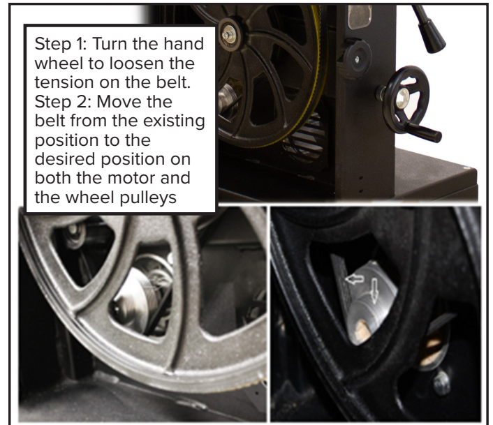
Figure 30: Changing the Band Saw Speed.
