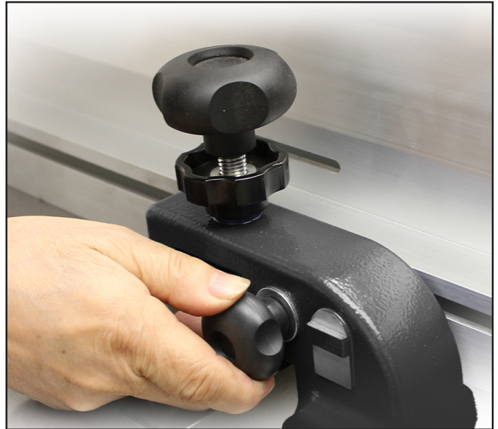
Figure 11: Securing the Rip Fence.
