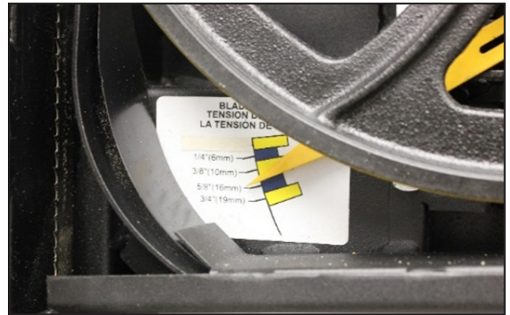
Figure 17: adjusting the pointer position.
