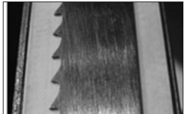
Figure 18: Tracking the blade.
