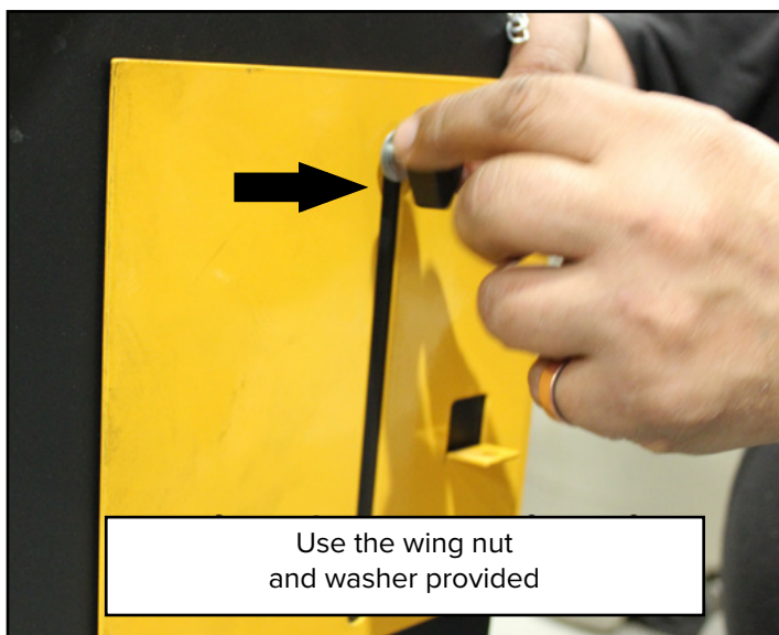
Figure 8: Installing the lower Blade Guard.
