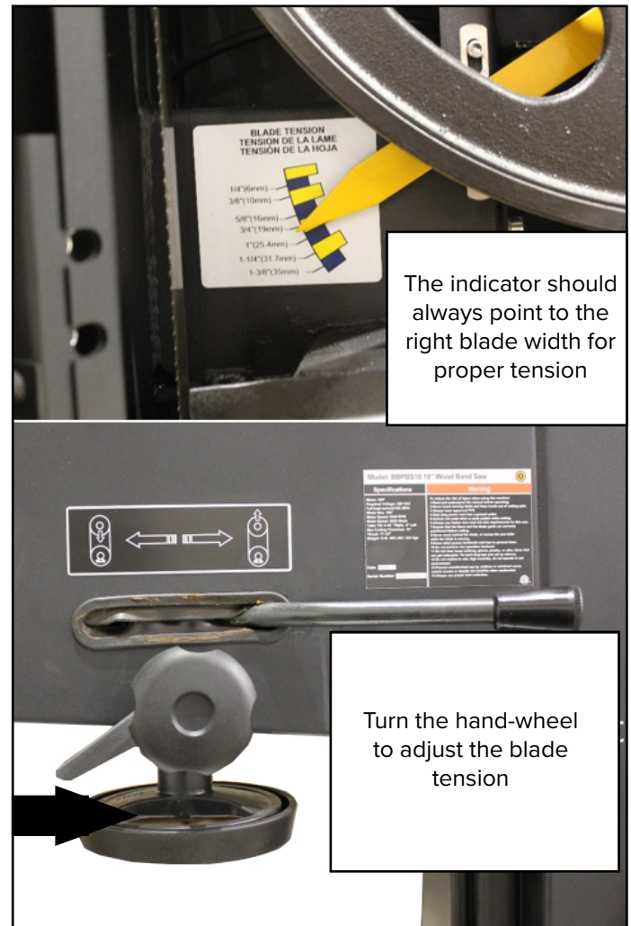
Figure 13: Adjusting the Blade Tension.
