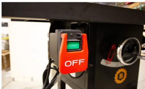
Figure 17: Positioning the switch on the front rail.
