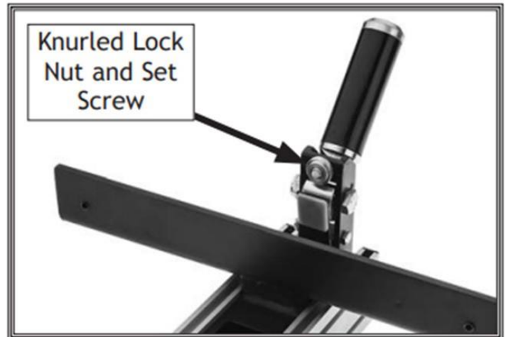
Figure 60: Fence lock handle adjustment.
