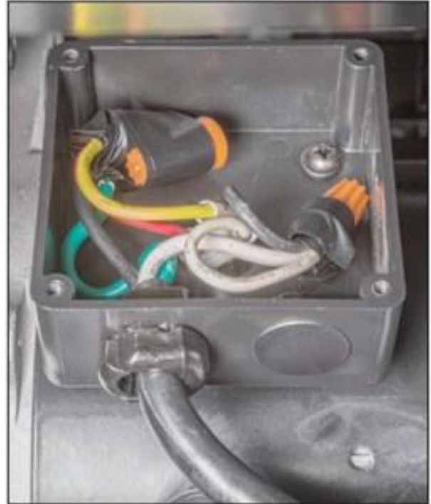
Figure 68: motor junction box.
