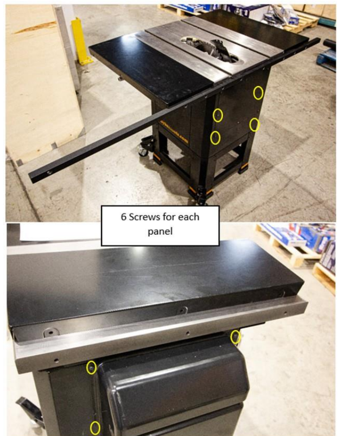
Figure 27: Installing the motor and rear access panels..
