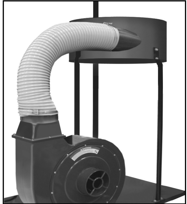
Figure-9 Connecting the hose from the outlet connector to the collector ring
