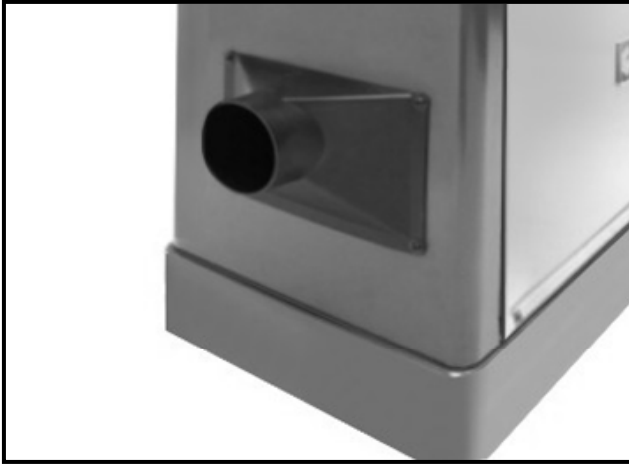
Figure-11 Installing the dust hood
