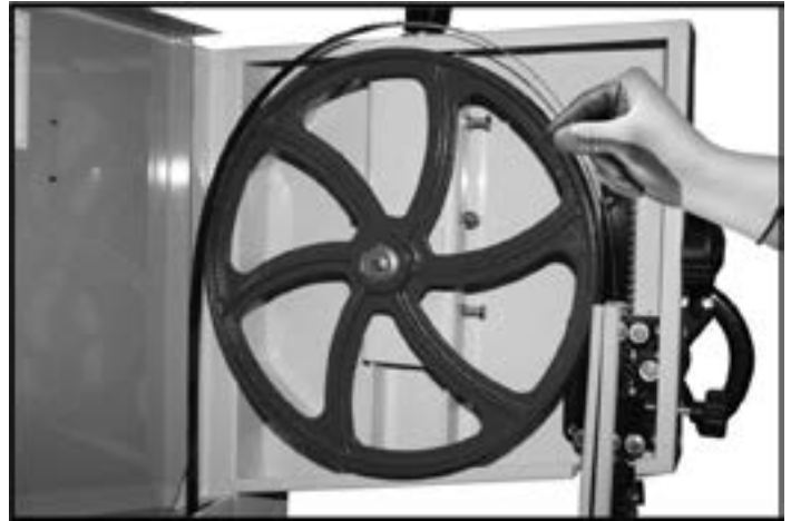
Figure-34 Installing the new blade
