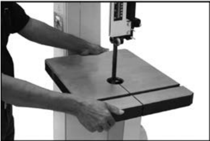
Figure-5 Installing the table
