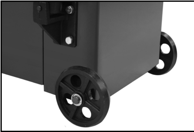
Figure-4 Installing the wheels
