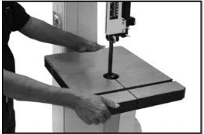
Figure-6 Installing the table
