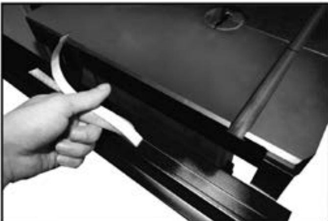
Figure-12 Adhesive backed scale attached to the front rail
