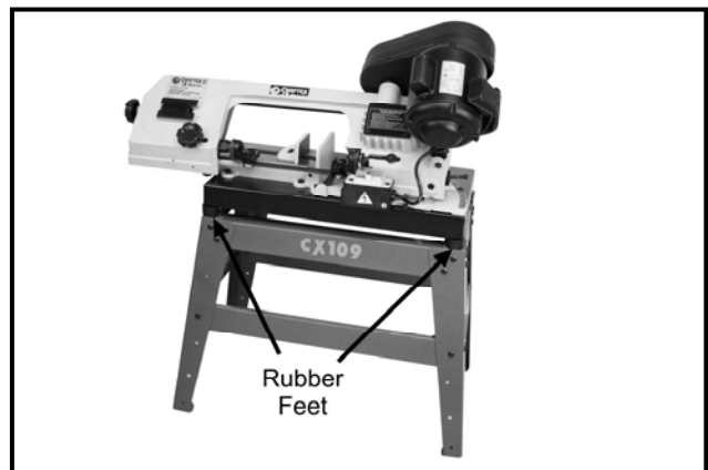
Figure-6 Installing the band saw onto the stand
