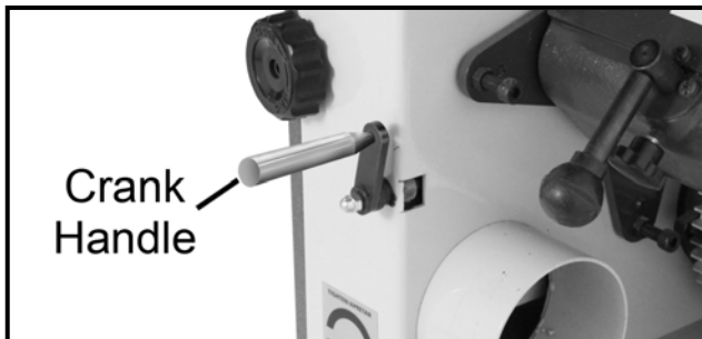
Figure-7 Installing the belt tensioning crank handle
