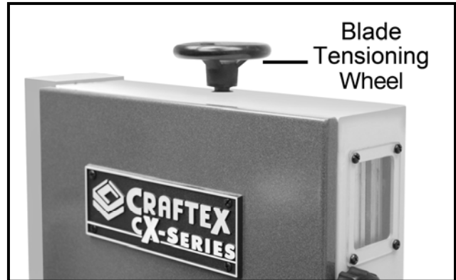
Figure-21 Blade tensioning Knob
