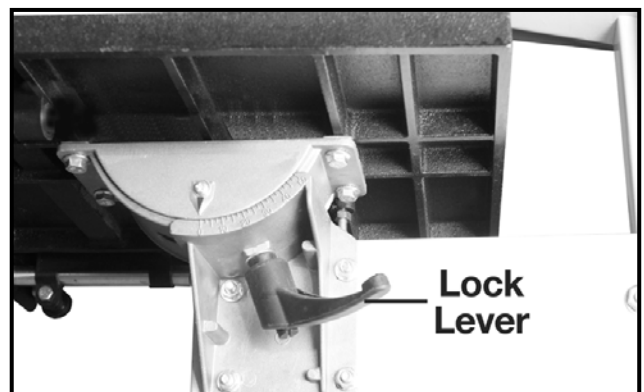
Figure-4 Installing the table
