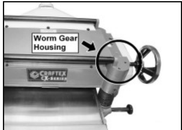
Figure-24 Worm gear lubrication location
