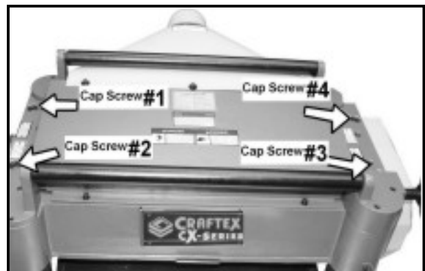
Figure-22 Set screws for the roller spring tension adjustment
