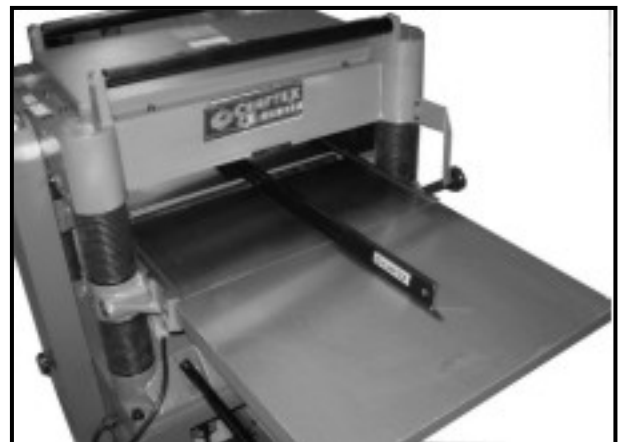
Figure-7 Leveling the wings using straight edge
