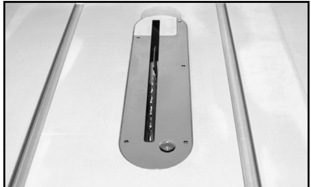
Figure-10 Installing the table insert
