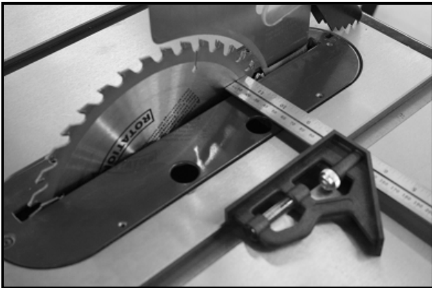
Figure-18 Measuring the distance using an adjustable square
