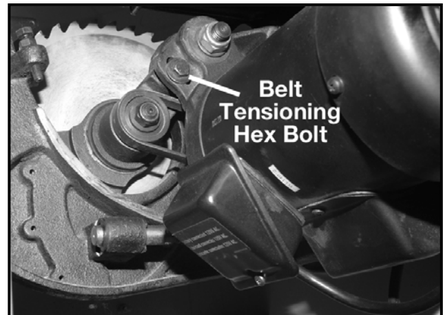
Figure-19 Belt tensioning hex bolt
