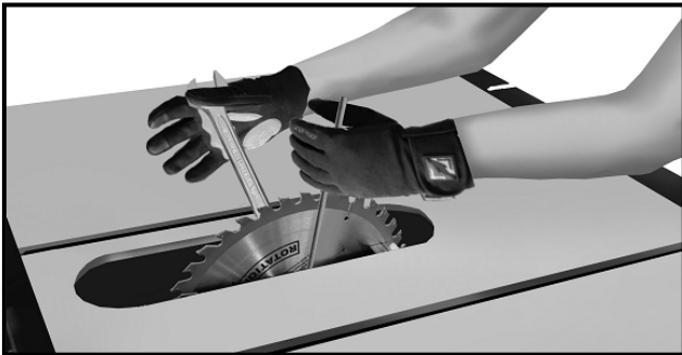
Figure-15 Installing the blade
