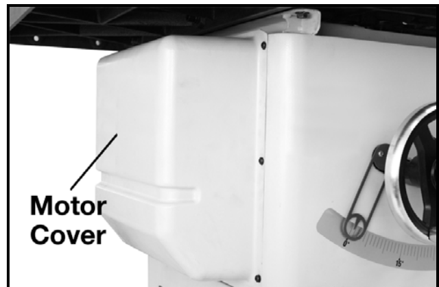
Figure-4 Installing the motor cover
