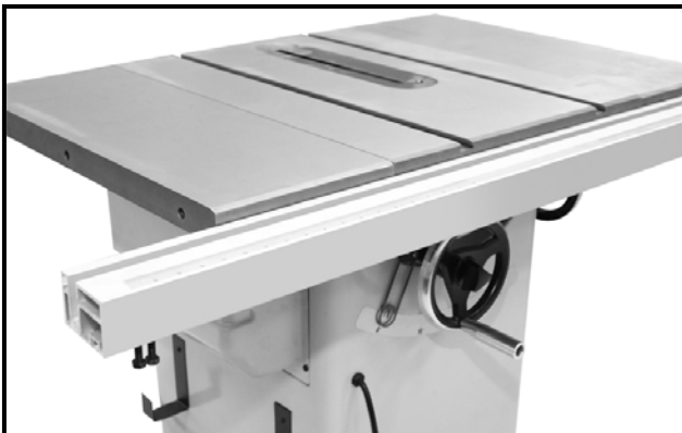
Figure-8 Installing the front fence rail
