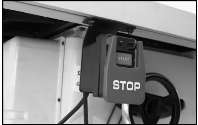
Figure-8 Installing the switch
