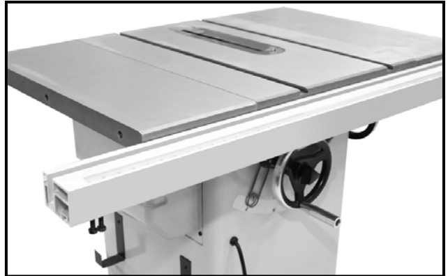
Figure-3 Installing the front fence rail
