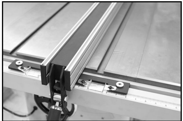
Figure-7 Scale installed on the front rail
