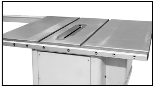
Figure-4 Installing the rear fence rail
