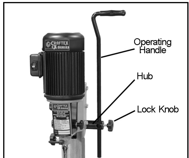
Figure-3 Installing the operating lever
