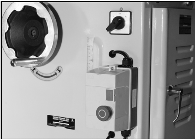
Figure-14 ON/OFF and Forward/Reverse Switches
