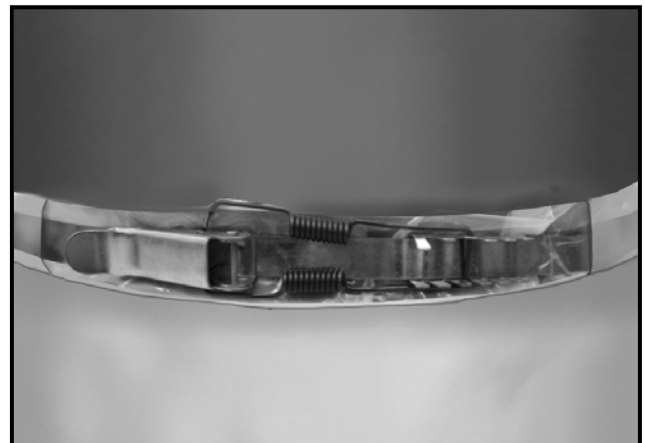
Figure-10 Installing the bottom bag
