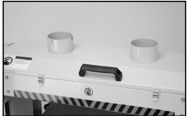
Figure-10 Dust ports on CX504
