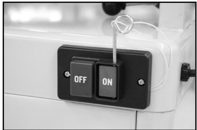
Figure-13 ON/OFF switch
