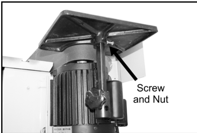
Figure-10 Installing the table onto the rod
