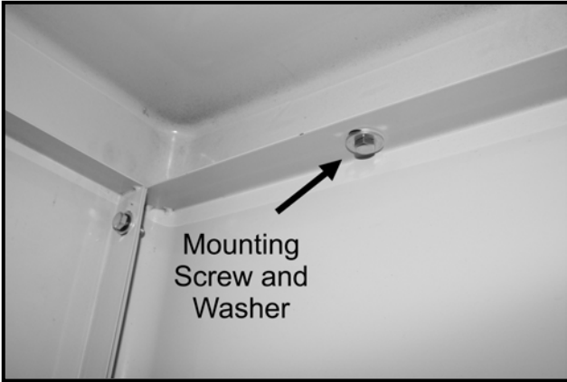
Figure-5 Securing the sander onto the stand from inside the cabinet
