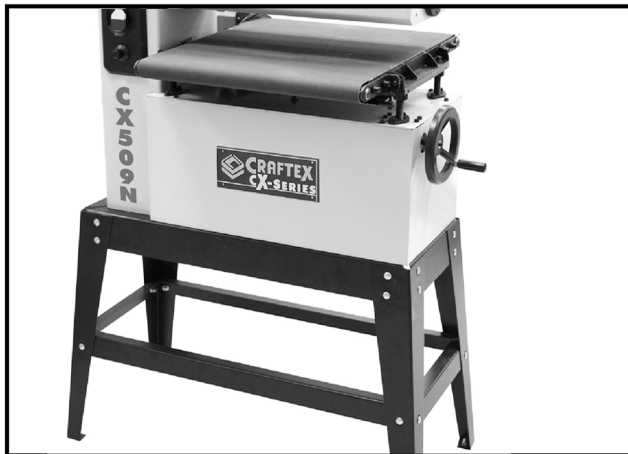
Figure-4 Securing the sander to stand
