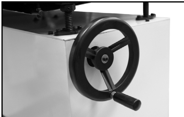
Figure-5 Installing the table height hand wheel
