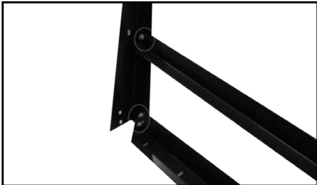
Figure-2 Attaching top and bottom long brackets to the stand leg
