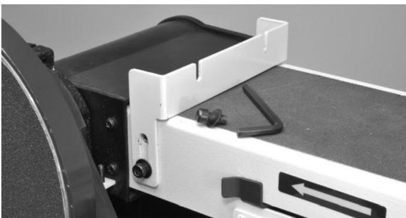
**Figure 2 – Install the small fence.**
