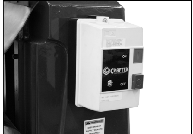
Figure-7 Switch box
