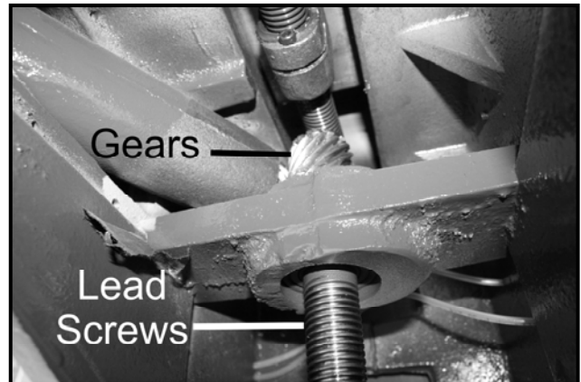
Figure-23 Lubrication bevel gears and vertical lead screws
