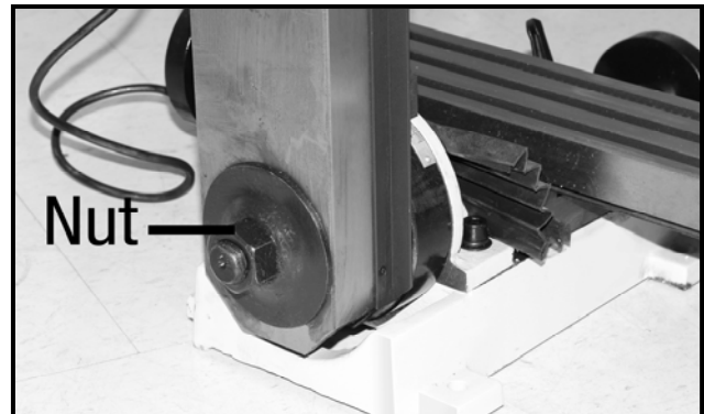
Figure-9 Loosening the nut securing the column to the base
