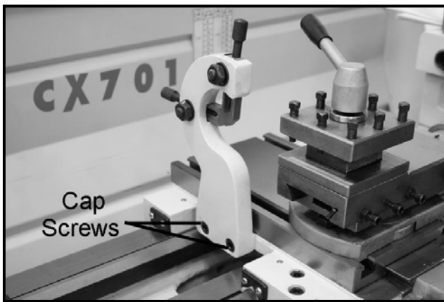
Figure-6 Follow rest installed
