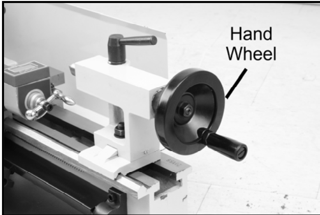
Figure-2 Installing the tailstock hand wheel handle
