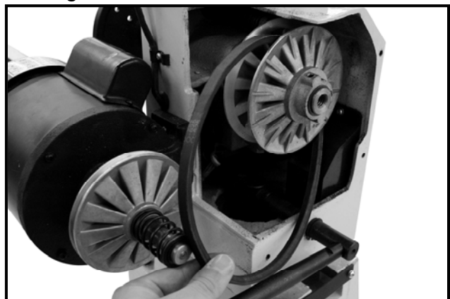
Figure-17 Removing the belt from the pulleys
