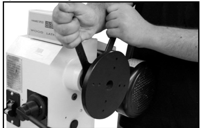
Figure-13 Installing the faceplate
