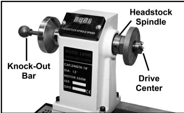
Figure-5 Knocking out the drive center with the help of knock-out bar
