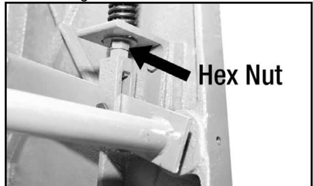
Figure-9 Return spring tension
