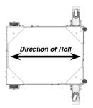
A short narrow base, such as found on a drill press or bandsaw, may benefit from this arrangement. Due to swivel rotation base may sit out of level. Rotate swivel wheel away from base to correct.
