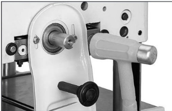
Figure H. Unseating cutterhead from tailstock.
