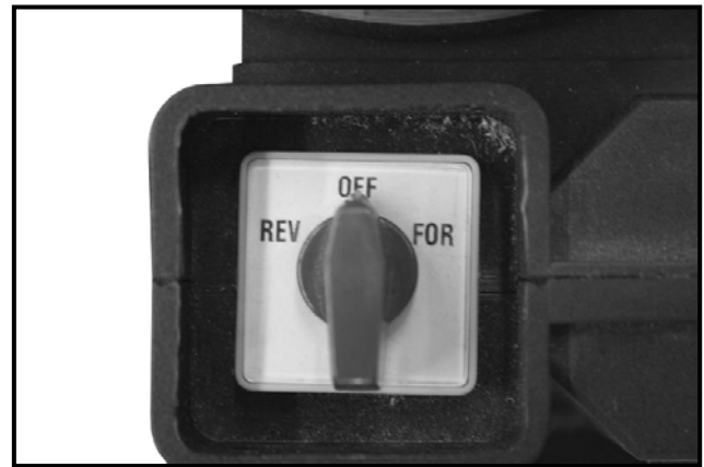
Figure-6 Forward/reverse switch in the OFF position
