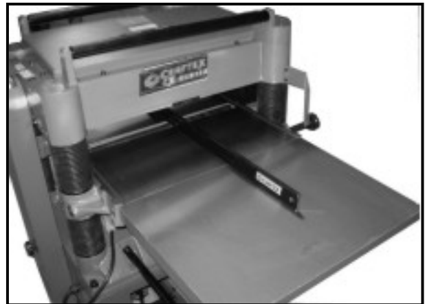
Figure-7 Leveling the wings using straight edge
