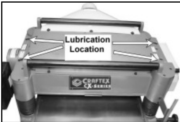
Figure-23 Lubrication holes for the feed rollers
