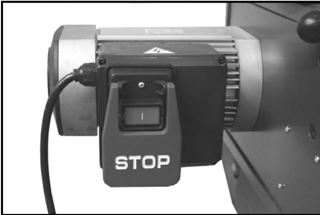
Figure-11 On/Off Switch
